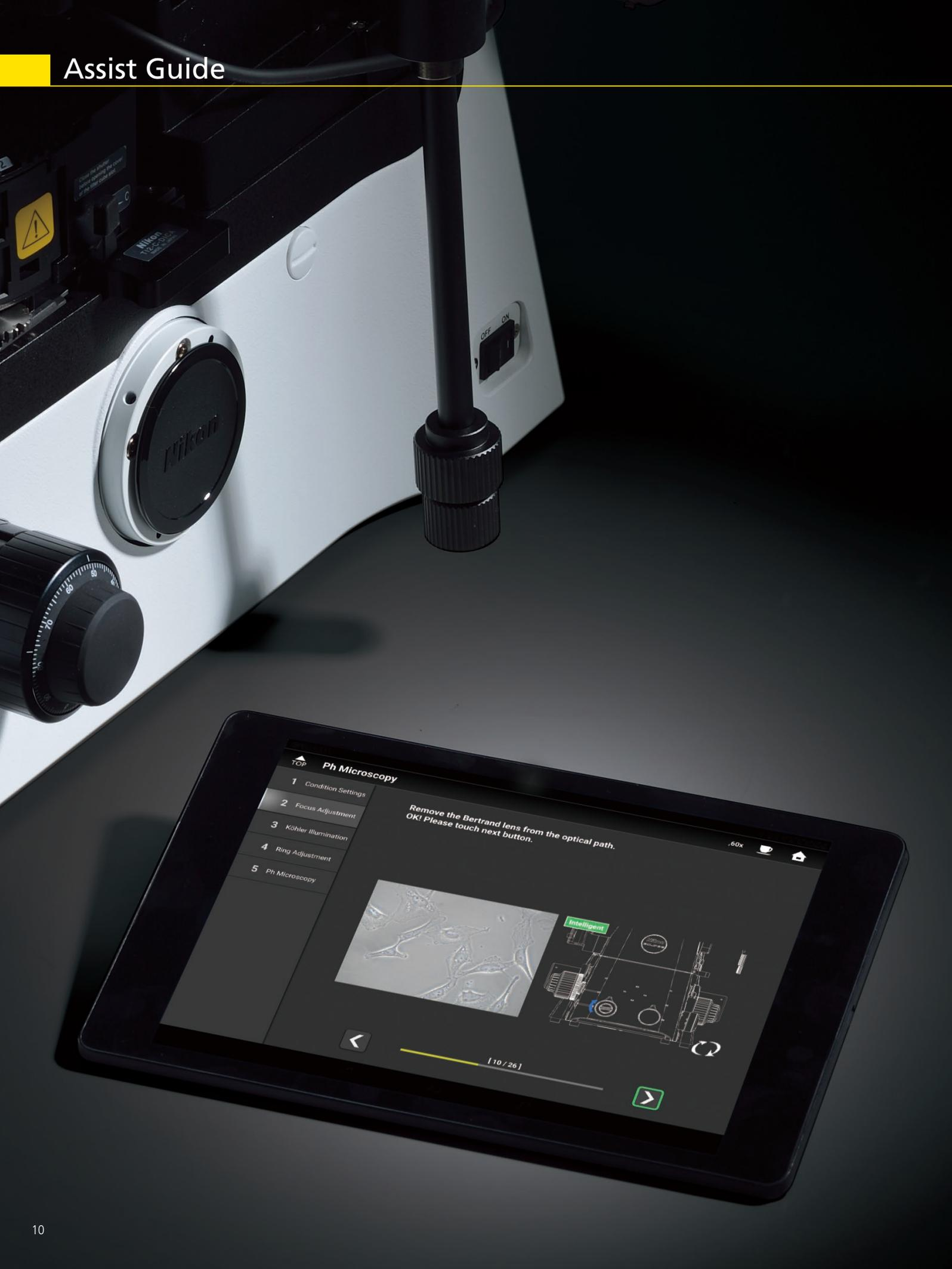
It is no longer necessary to memorize complex microscope alignment and operation procedures. The Ti2 integrates data from sensors to guide you through these steps, eliminating user error and enabling researchers to concentrate on their data.
